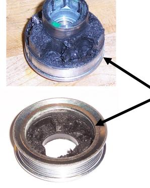
The damping elements within this part lasted only minutes prior to heat damage. Elements were completely melted.
